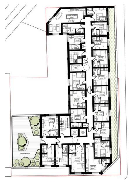
Proposed Third Floor Layout – this plan demonstrates 5 x cluster units located at the northern part of the site and 14 x studio units on the central and southen part of this floor. There is a third floor terrace located on the western side of the site.
